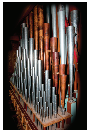
J. W. Walker & Sons 1984 3 manuals, 56 ranks 40 stops, 3,056 pipes Mechanical Action
